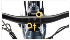
Attach the handlebar to the stem bar. When attaching the screws, insert two screws diagonally first to make sure each screw is aligned, then screw on the rest.
