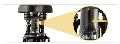
Install the seat onto the seat post.
