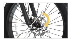
Tighten the screws with washers on both sides to complete the installation.
