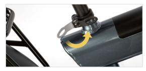
Loosen and tighten the saddle clamp to adjust the seat according to your height.
