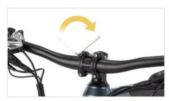
Adjust the LED Screen to a comfortable position and tighten all 2 bolts.
