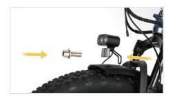
Align the front light with the installation position of the front fork. Adjust to the appropriate angle and tighten the screws to complete the headlight
