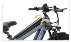
When removing the battery, turn the lock key to losen the battery.
