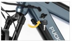
Once the battery is released, turn the key while holding the battery. Then remove the battery by lifting the top part first.
