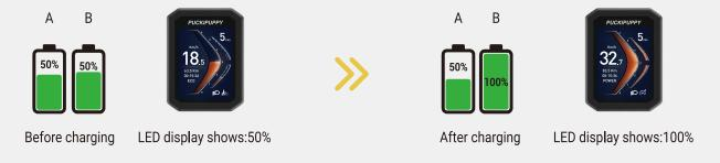
When both A and B batteries have 50% charge left, the display will show an overall charge of 50%. At this point, if Battery B is charged to 100% and reinstalled, the display will show 100% (The display will prioritize the battery with the higher percentage charge remaining). And this time will preferentially consume the power of battery B.
