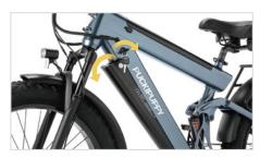
Similarly, when the other battery is removed, turn the locking key to release the battery.
