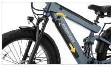
Insert the bottom of the battery into the socket first, then press the top part of the battery down to secure it (it will make a clicking sound).
